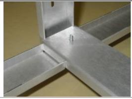
The next step is to slip the mated Aft Leg/Angle Bracket pair down onto the 6-32 stud in the center of the Front Leg so that the 6-32 stud protrudes up through the aligned holes in the Aft Leg/Angle Bracket. Note that the open section of the Front Leg is oriented upwards (opposite orientation of the Aft Leg) to interlock with the Aft Leg/Angle Bracket assembly. Attach (1) Knob to the 6-32 stud and tighten securely.
