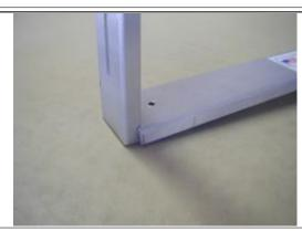
The first step is to mate the Aft Leg to the Angle Bracket. Note the Aft Leg interlocks into notches in the rear of the Angle Bracket as shown. When fitted properly, the hole in the Aft Leg and the the hole in the Angle Bracket will coincide.
