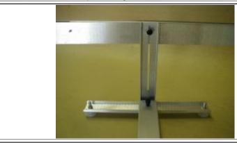
Remove the knob attaching the Scale Bracket to the Angle Bracket, rotate the Scale Bracket 90 degrees, and re-attach the Scale Bracket to the Angle Bracket using the 6-32 stud located in the center of the Scale Bracket.
