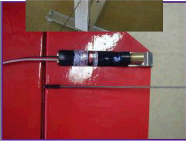
Step 3) To ensure maximum accuracy, make sure the Laser Clip is oriented approximately 90 degrees to the control surface hinge line.
