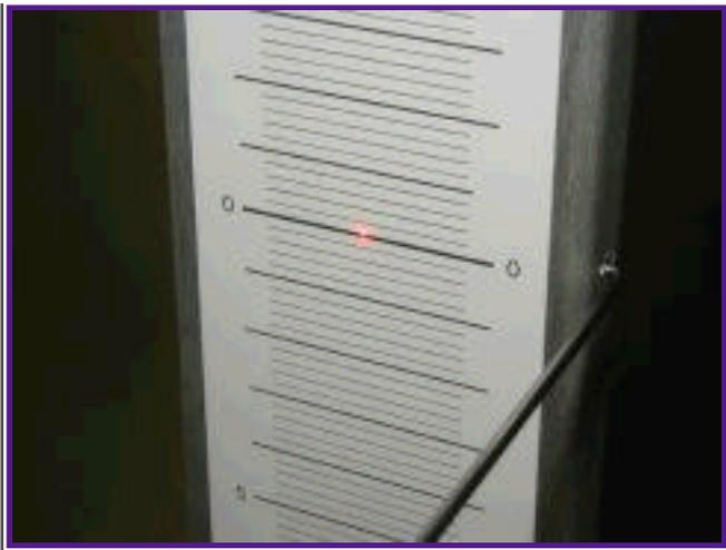
Step 4) Loosen the Knob on the back of the Scale Bracket and adjust the vertical position of the Scale Bracket until the Laser Beam is centered on the 0 degree mark.
