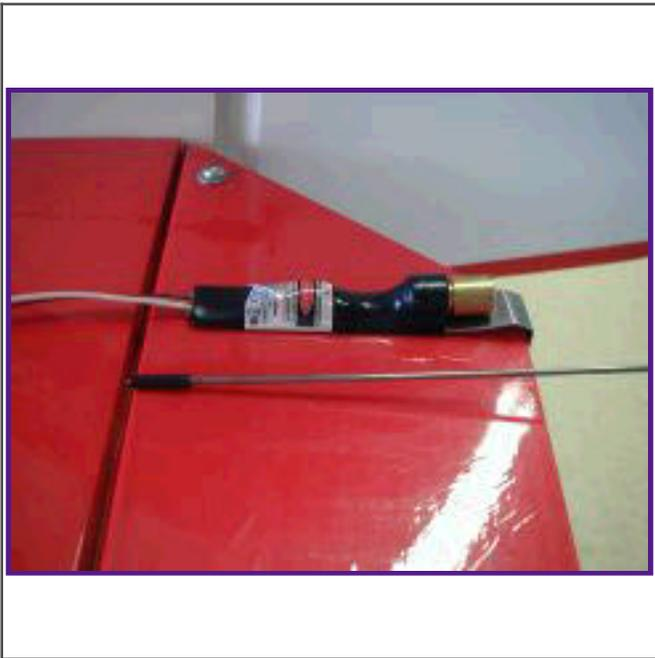
Step 2) Mount the Laser Clip onto the control surface and locate the wire position indicator immediately adjacent to the Laser Clip so that the rubber tip is aligned with the hinge line of the control surface. Plug the Laser Clip into a battery source (4.8v to 7.2v) and select the appropriate light intensity with the slide switch ("Off" for outdoors, "On" for indoors). Turn on the transmitter and airborne R/C system and center the control stick.
