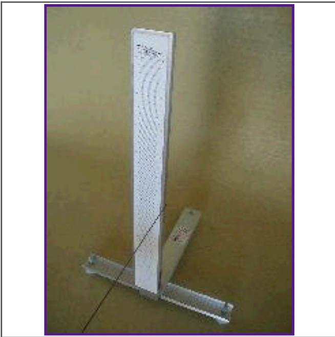
Step 1) To use the Laser measurement System remove the wire position indicator from the top hole in the Scale Bracket and attach it to the middle position hole near the 0 degree indication mark on the Scale (see photo above).
