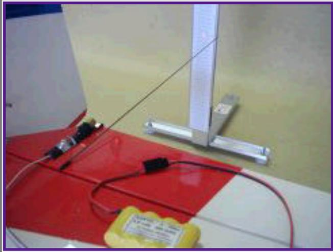
Step 6) Readjust the distance from the hinge line, the height adjustment of the Scale Bracket, and the height adjustment of the adjustable feet until all angles are ~90 degrees, and the Laser beam is positioned on the 0 degree mark. This may take several iterations to complete, but it will ensure the accuracy of the measurement. It is not important that the system be level, only that the specified angles are ~90 degrees.
