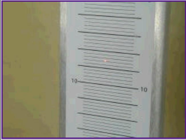
Step 7) Move the control stick to it's positive and negative position limits and observe the corresponding control surface deflections on the Measurement Scale. In this example the surface deflection is +11.45 degrees.
